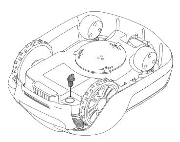
Insert the safety key into the underside of mower and turn to the  $\ensuremath{\textbf{Enable}}$  position.
