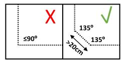
Do not lay the guide wire at sharp angles or the mower will have difficulty following it.
