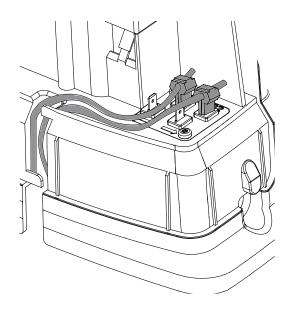
Installing a second guide wire
