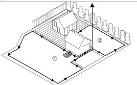
Temporarily secure the end of the loop wire to a peg or other object at the charging station.
