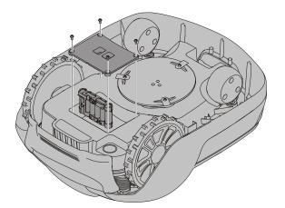
WARNING! Press the STOP button and remove the safety key before replacing batteries and wear protective gloves. CAUTION: Use only original replacement parts.
